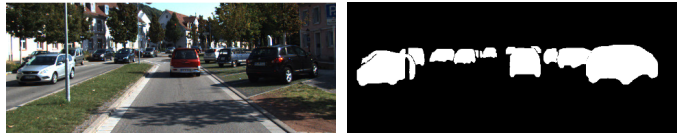
Fig. 4: An example of object mask generated using a pre-trained Mask-RCNN [58] on left image sequence 000123_10 of KITTI 2015 [16] stereo dataset.
